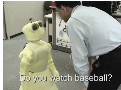
図 12 A scene from the experiment. A person is communicating with Robovie-IV. The robot is asking if the person watches a baseball game.
